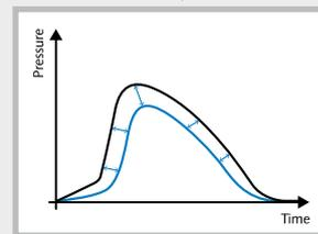
2 Analysis of deviations between current measurement and reference. This is the basis for a specific suggestion on adapting the machine parameters.
