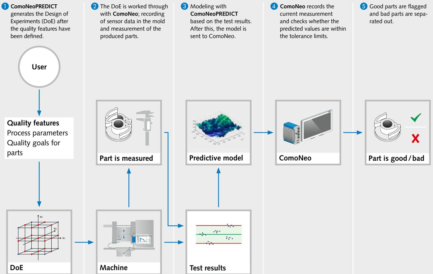
In the second step, the DoE is worked through with ComoNeo on the injection molding machine; all cavity pressure curves are recorded and the parts are removed and measured. Features such as surface quality or flash can also be evaluated. Then the results are fed into the ComoNeoPREDICT software and linked to the mold measurements (pressure, temperature). The software uses this data to produce a model so that part quality can be predicted on the basis of the mold measurements.
