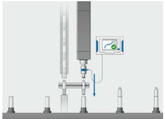
Process monitoring on an insulin pen production line: quality assurance underpinned by process-integrated inspection and documentation
